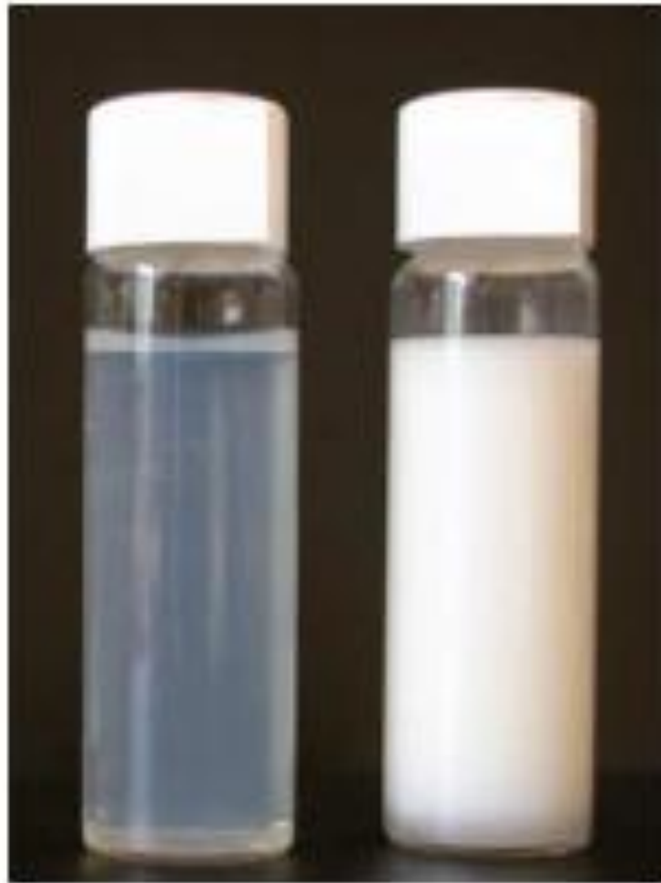
Fig. 1. Picture of a nano-emulsion (left) and a macro-emulsion (right) with droplet diameters of 35 nm and 1 \mu\text{m} , respectively.
